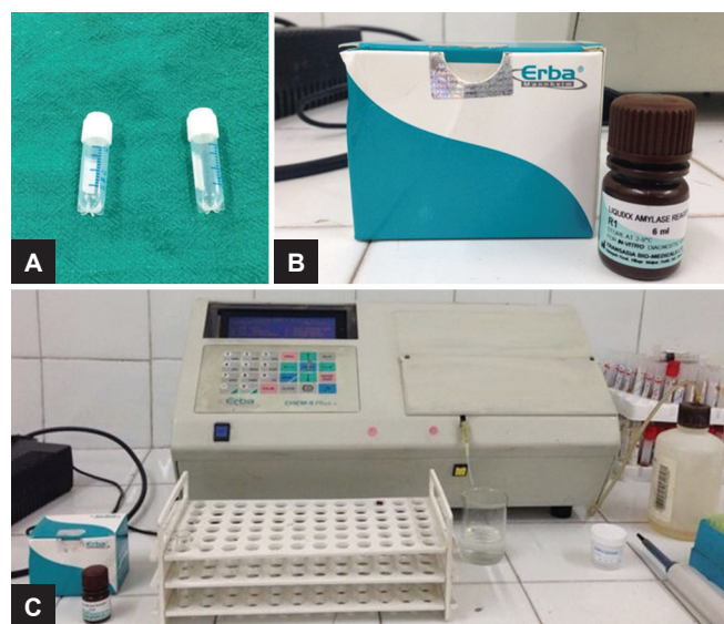
Figs 1A to C: (A) Fasting and postprandial salivary samples; (B) salivary amylase reagent (Erba); and (C) semiautomatic analyzer for salivary amylase estimation (Erba)
