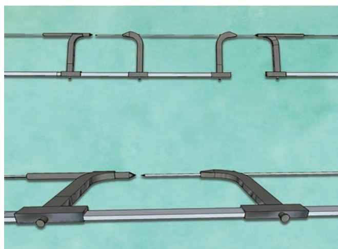
Fig. 2: Suggested conception of a tunnel aimer that keeps the femoral and tibial tunnel in one axis. All four movable aimers slide on a metallic band to keep all aimers in one line and ensure that the guide wires pass from tibia to femur or from femur to tibia in one line
